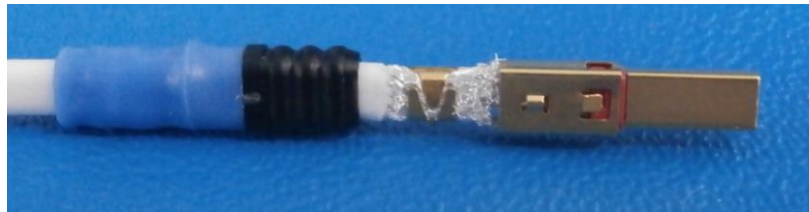
Figure 13: Crimped strain relief
