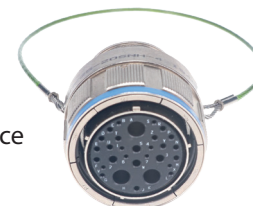
Retraction of the lanyard sleeve allows the threaded coupler—split into six sections—to rapidly expand and release.
