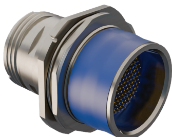
253-034 bulkhead feedthru with misalignment accommodation, float-mount jam-nut to D38999-type receptacle
