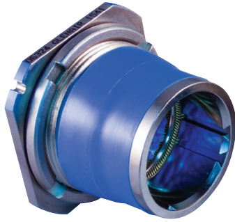
253-028-07 fixed jam-nut panel-mount PC tail receptacle with misalignment accommodation and external environmental seal
