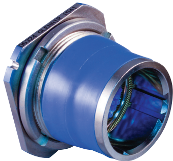
253-045 high-speed float-mount receptacle series with chamfered nose, misalignment accommodation, and external environmental seal
