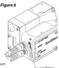
Caution: Adjusting cut-off delay timing too short will result in premature cut-off, and a loose clamp.
