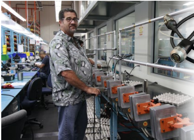
◀ Special-purpose overmold tooling and fixtures for small form-factor sealed Mighty Mouse cable assemblies
