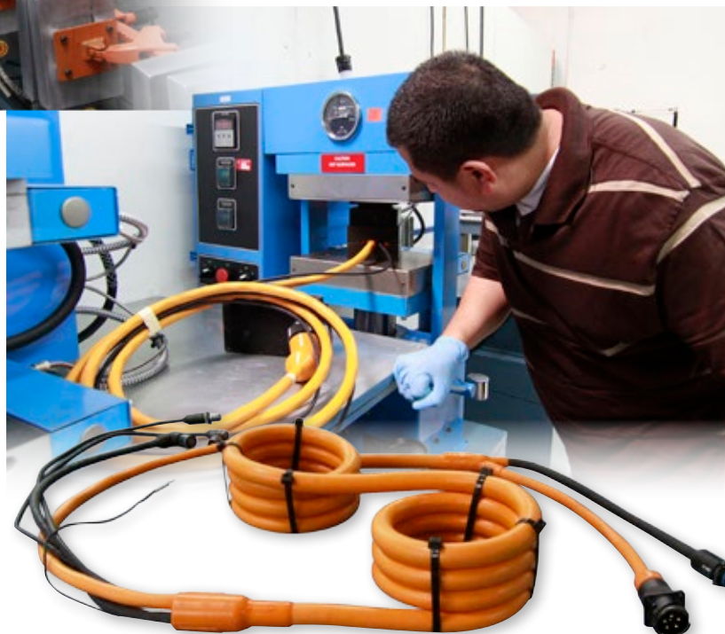
▶ High-volume production overmold and cable encapsulation tooling and equipment for Duralectric™ cable assemblies
